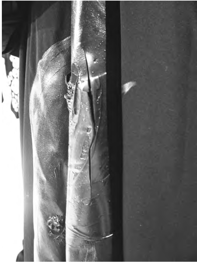
Figure 3 Detail of damage to PVC appliqué: large splits occurring in surface
