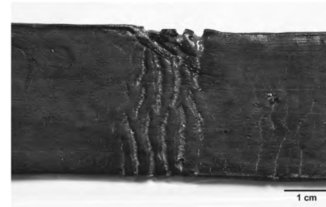
Figure 2 Details of PUR elastomer rings with signs of material deterioration and loss of plasticisers. © Hamburger Kunsthalle, photo: Julia Langenbacher.
