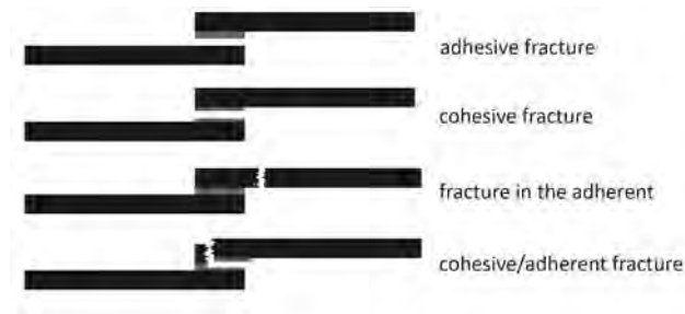
Figure 6 Schematic illustration of failure patterns
