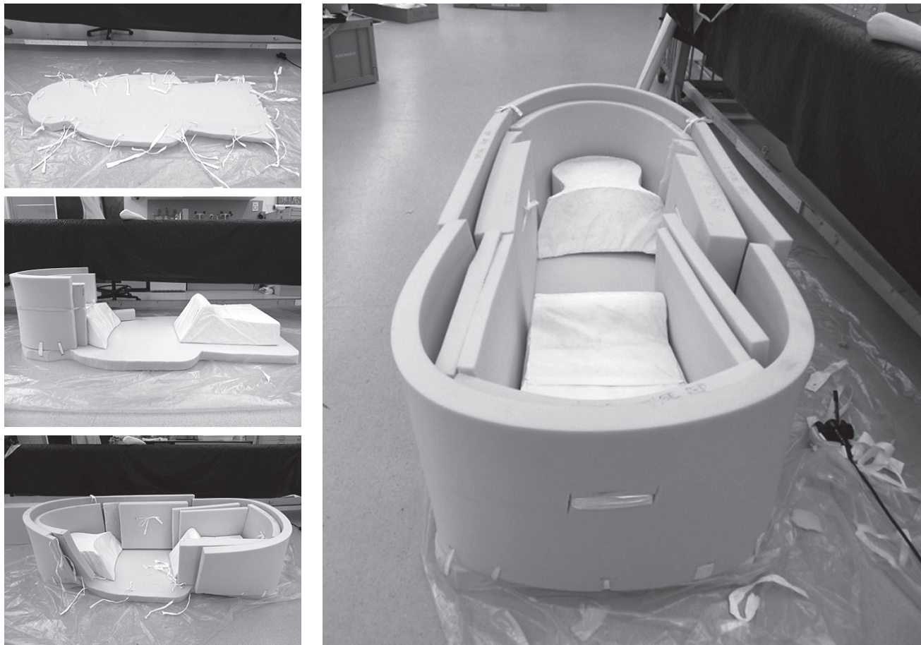
Figure 5 The reconstruction of the padding made by Ferdi (prototype model) before it was built piece by piece into Wombtomb's upholstery. Photos: Anna Lagana
