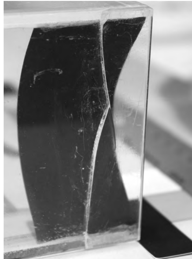
Figure 4 Area around the breakage before and after the removal of the adhesive layers.
