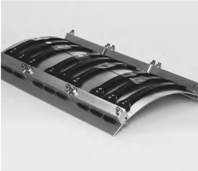
Figure 4 Bent-beam method. Test specimens in the bending template coated with adhesive and covered with plastic sheet.
