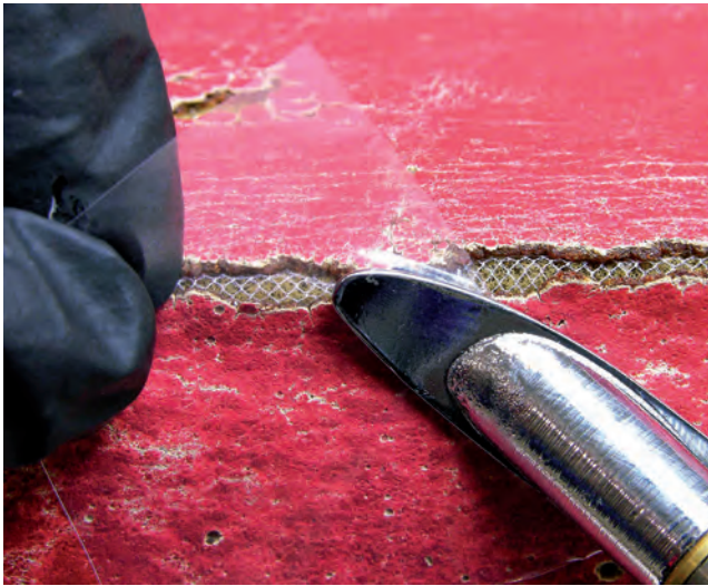
Lecture 005 / Figure 2 Conservation treatments – consolidation of the coating, securing the edges of the coating with synthetic netting, reshaping of the deformed edges of the coating, filling losses in the foam body with inlays
