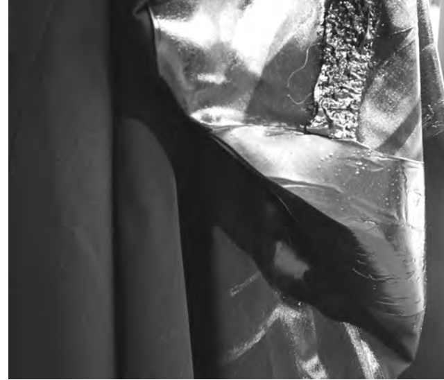
Figure 5 Detail of damage to PVC appliqué: surface becomes tackier and 'flowing', causing distortions
