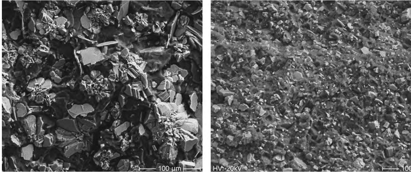
Figure 4 Back scattered electron microscopic images of (a) the solid Corian® surface (sample 1, left) and (b) of Corian® joint adhesive (sample 3, right). Photographs were taken at 20kV.
