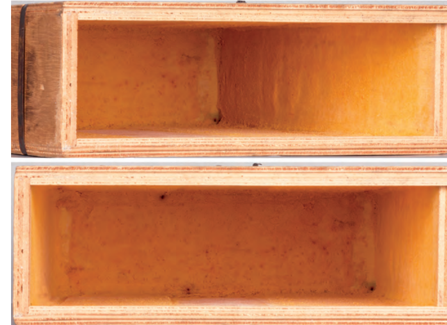
Poster 004 / Figure 5 a) bottom/side view of the inside of the plywood slipcase after treatment; b) bottom view after treatment; c) detail of polyester urethane foam with consolidated fragment.
