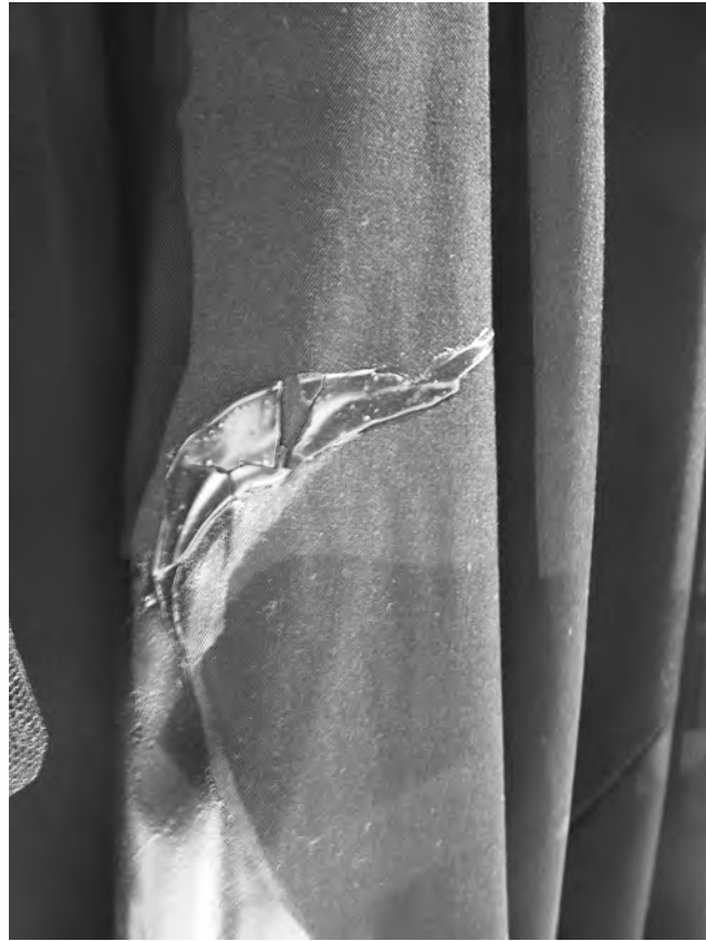
Figure 4 Detail of damage to PVC appliqué: surface lifting and adhesion to cotton surface failing, leaving areas of loss
