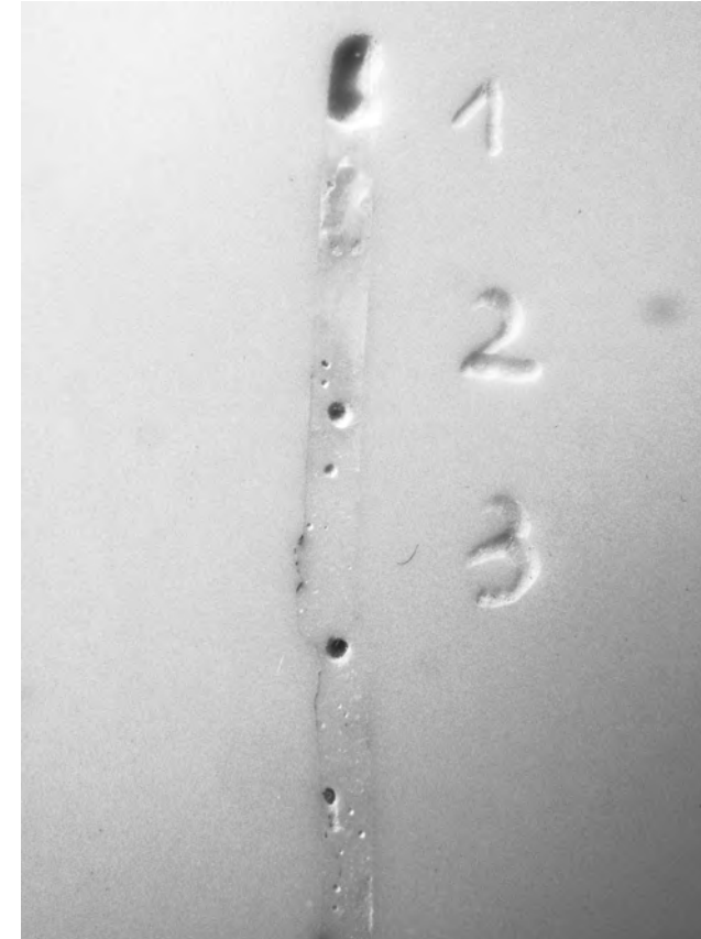
Figure 5 Putties based on Corian® adhesive modified with ATH, grinding blades and/or powdered Corian®.
