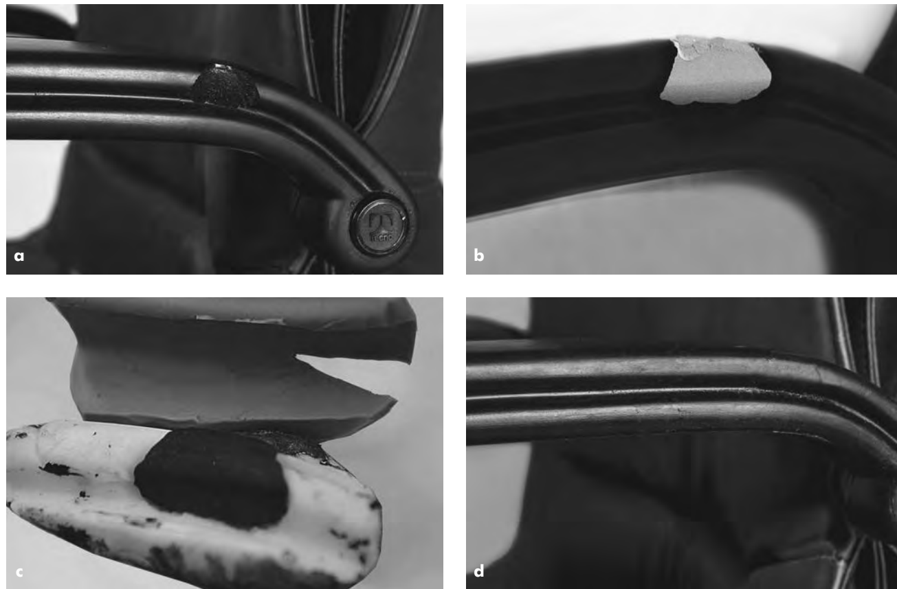
Figure 4 Treatment phases of Qualis a) Photograph of the polyurethane gap damage b) Testing the into the prepared model casts c) Model made of Sintagom Neutro into a small rubber mould 'bivalva' d) After treatment
