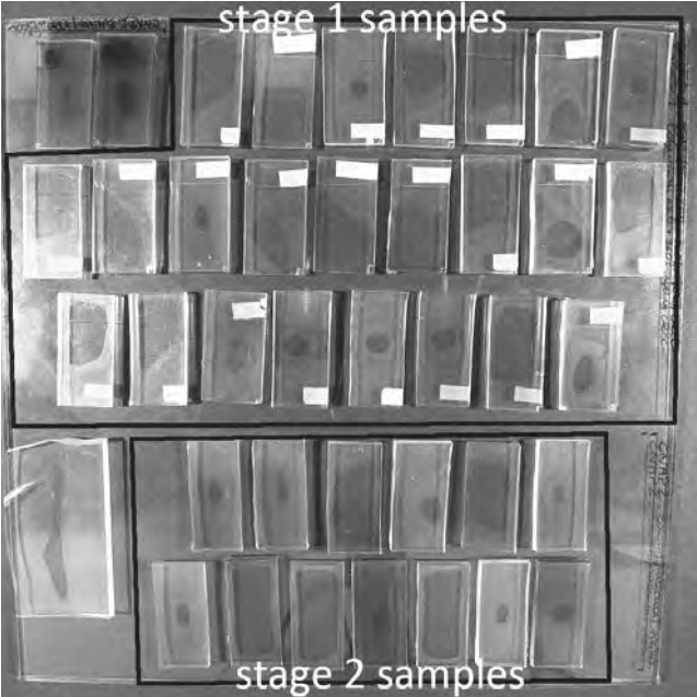
Figure 4 On the left side: stage 1 and stage 2 samples after artificial ageing. On the right side, tidelines left on the glass plate after removal of the samples. © Clémentine Bollard
