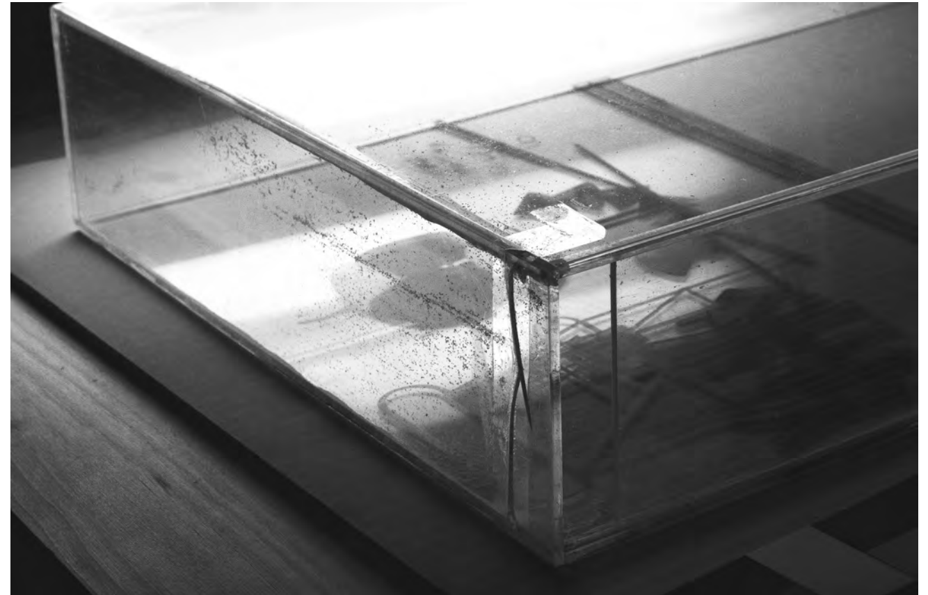
Figure 2 Breakage in the bottom sheet (here on the left side) with attached self adhesive tape.
