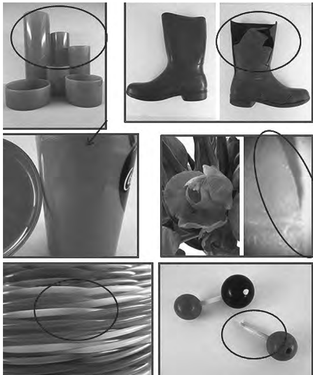
Figure 1 Objects from the Van Oosten reference collection showing discolouration (first 2 rows) and colour transfer from red to white plastic part (bottom row) (see colour plate, p. 162)
